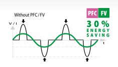
The GYSMI 200E FV has a powerful integrated PFC and features FLEXIBLE VOLTAGE (85-265V).
